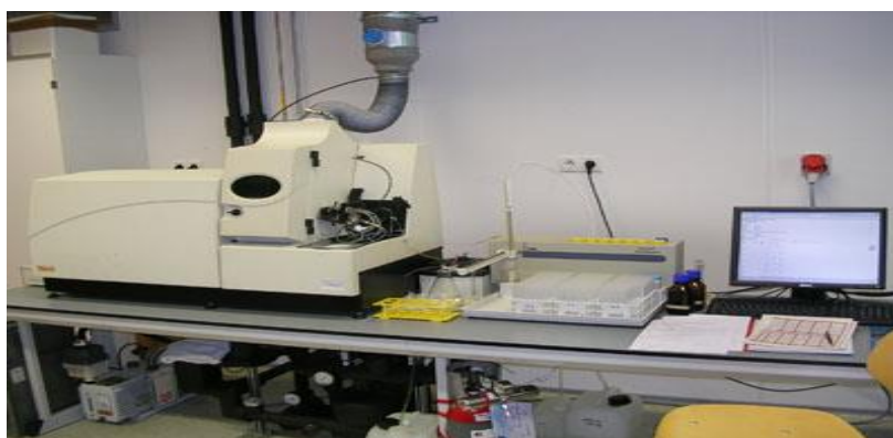
Figure 14: Inductively Coupled Plasma-Mass-Spectrometry (picture taken from Radboud University, Faculty of Science, General Instrumentation Department)
