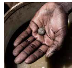
4. The gold is mixed with mercury, which forms a ball which will later be heated to extract the gold
