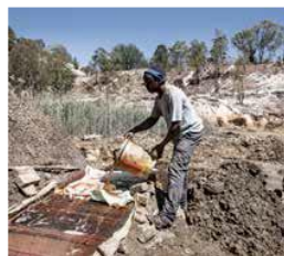
2. Water is then poured over the powder over towels, where heavier particles (including gold) are caught
