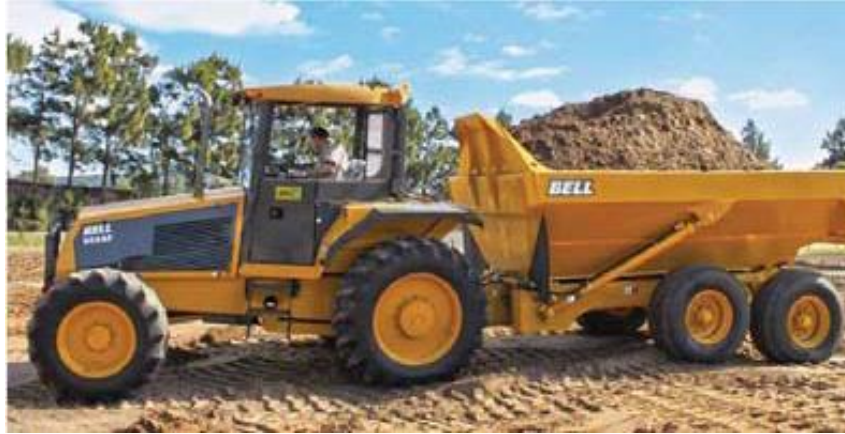
Figure 11: Tractor-Trailer arrangement (Bell, 2012)
