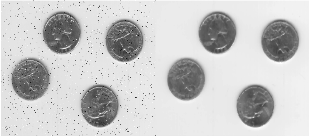
Fig. 4.1. Noise removal by using median filtering
