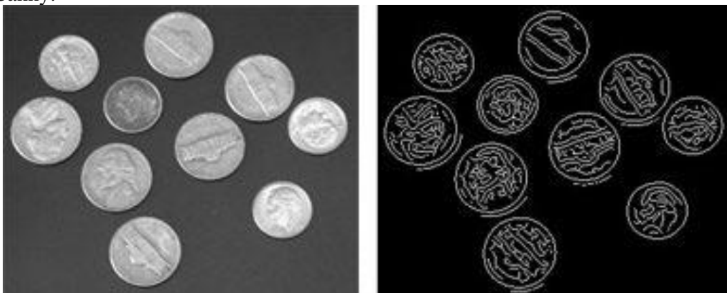
Fig. 4.2 Edge detection using the canny method
